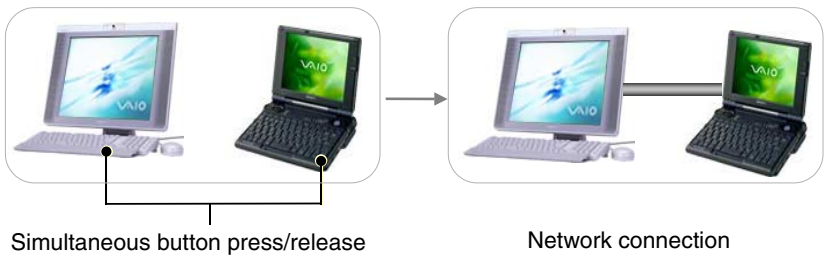
Fig. 1. SyncTap: user synchronously presses and releases the buttons on the devices, then these device establish a network communication
