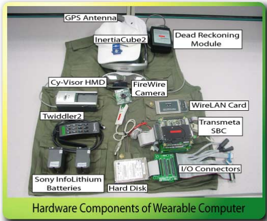
Fig. 2. Detail configuration of wearable computer
